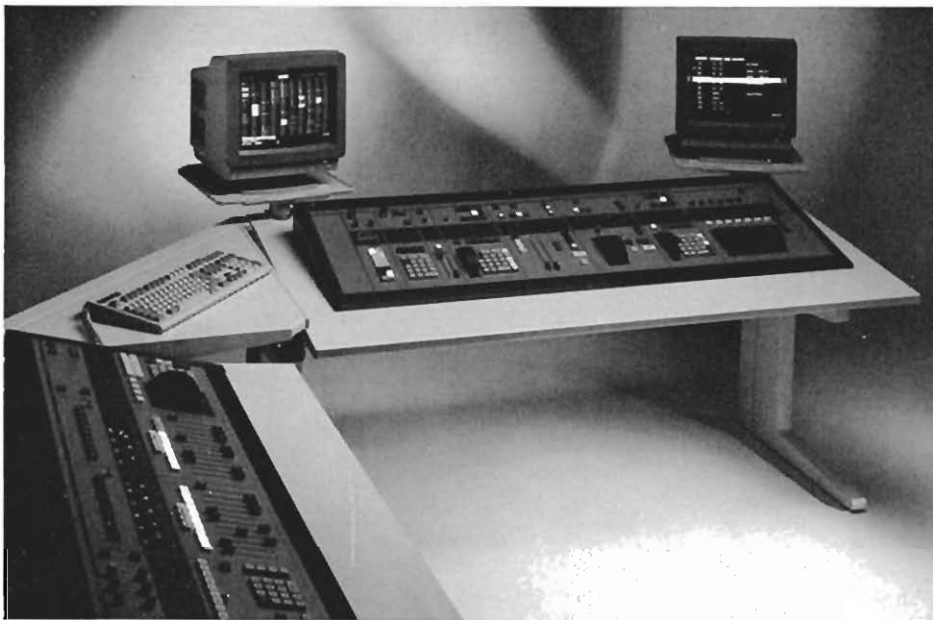
The big one - Galaxy 3 from Strand Lighting. Control of motorised luminaires is fully integrated into the operational structure.
