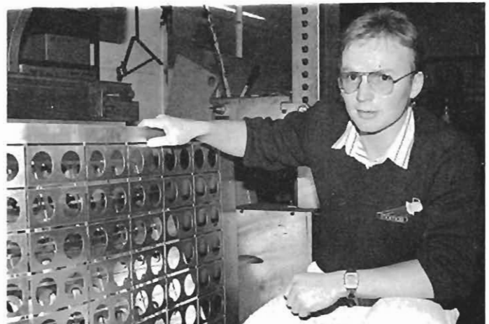
Mervyn Thomas with pressed sheet for 10-way Light Batters.
