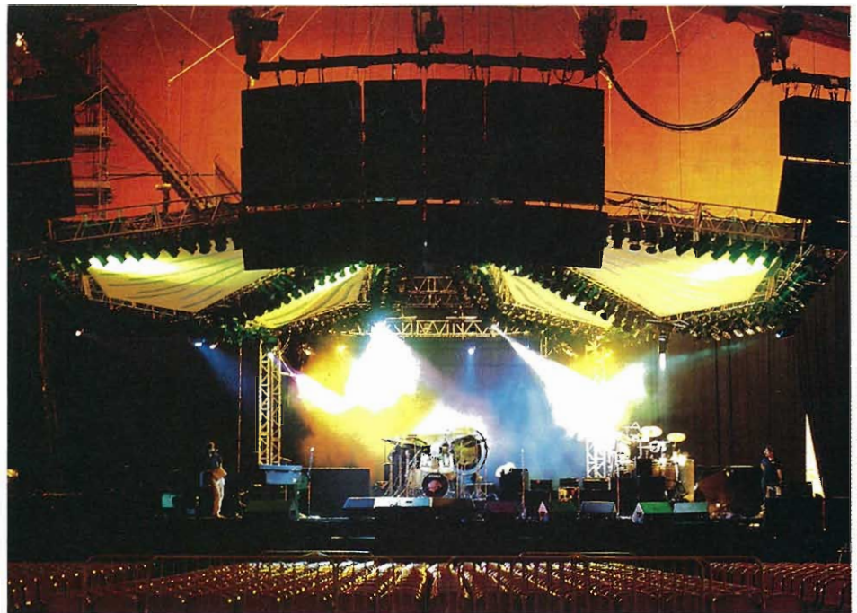
Fleetwood Mac, Wembley 1988. The Thomas pre-rigged truss was designed in the form of animated butterfly wings. Ground support towers can be seen at back of stage. Par cans are also Thomas.
